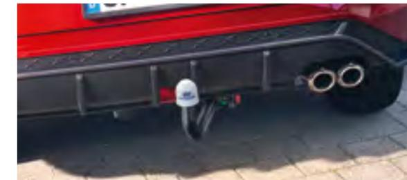
Enganche de remolque desmontable, BE281ADE00NL (N Line)
